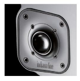
Diva tweeter is uncoupled from the enclosure through a soft rubber shell, which makes it a virtually "floating" component: in this way we obtain an important reduction of the vibrations sent from the cabinet to the tweeter. The proper excursion of the dome is controlled by a radial resonance chamber, provided with two different types of acoustic damper, vplaced under the dome and inside the venting ring.
