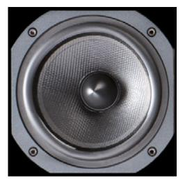
For the mid-woofer cones we chose the Curv: a rigid, light and damped material, made with pure polypropylene extruded, woven and heat treated. Furthermore, we have equipped the magnetic circuit with Aluring: an aluminium short circuit ring that reduces the non-linearity, which affects all the commonly made magnet systems, increasing the voice coil controlled excursion capability.
