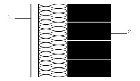
Sound Insulation R (db)= 60 dB 1. InsulMur 2. Perforated Brick
